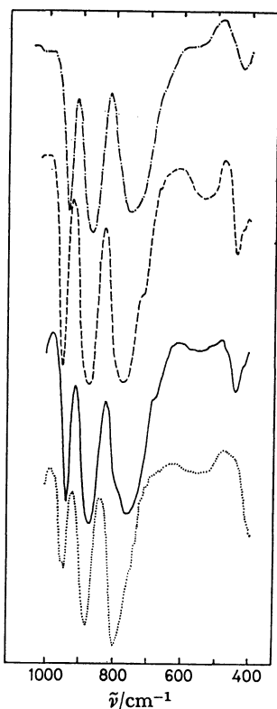
Fig. 1. IR spectra of tetrabutylammonium salts of MW_{12}O_{40} heteropolyanions in 1000–400 \text{cm}^{-1} region measured in KBr disk; semi-dashed line (---) for M=\text{Cu}^{\text{II}} , dashed line (-----) for M=\text{Fe}^{\text{III}} , full line (—) for M=\text{Co}^{\text{II}} and dotted line (.....) for metatungstate.
